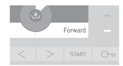
Press button Open the door O= (is not lit!). The programme will be interrupted and the door unlocked.
