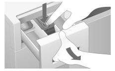
Press down the blue tab in the compartment ( and pull the drawer all the way out.
