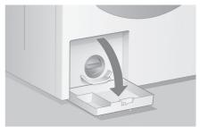
Open the maintenance hatch at the machine front.
